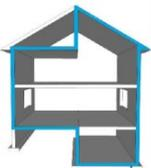
The highly energy-efficient envelope protects against thermal bridging and moisture problems in a hot, humid climate. Testing showed air leakage is 75% less (better) than the standard.<sup>1</sup>
